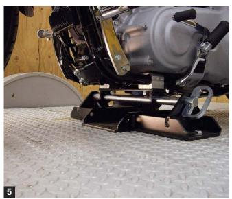
Slide the locking pin through the Frame Lock and the eyelet bracket. Use a cotter pin or padlock to lock the pin in place. If the holes do not line up properly, you may not be centered over the Frame Lock.
